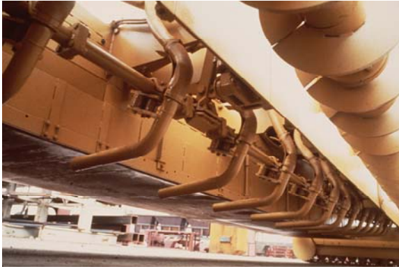
Figure 8.5 –Vibrator layout and position
